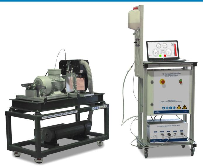
Equipment designed for the study and understanding of the behavior of a four-stroke single cylinder diesel combustion engine.
